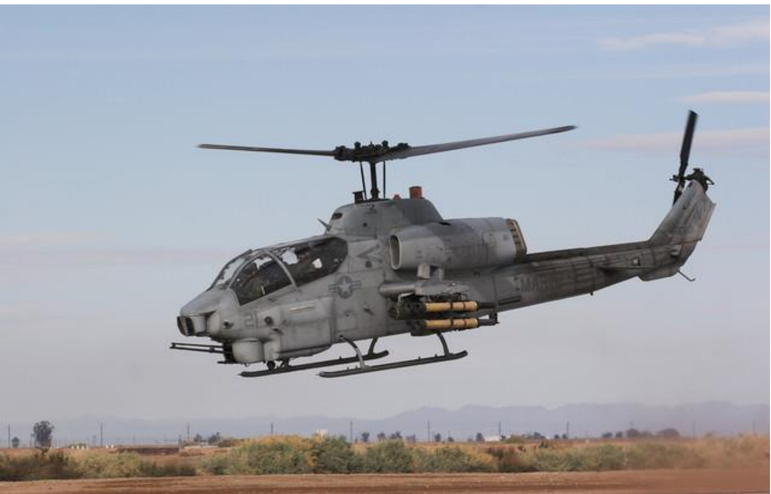
Light Fire Team Helicopter. Bell AH-1 Cobra Gunship , with forward protruding Mini-Gun and side mounted rockets.
