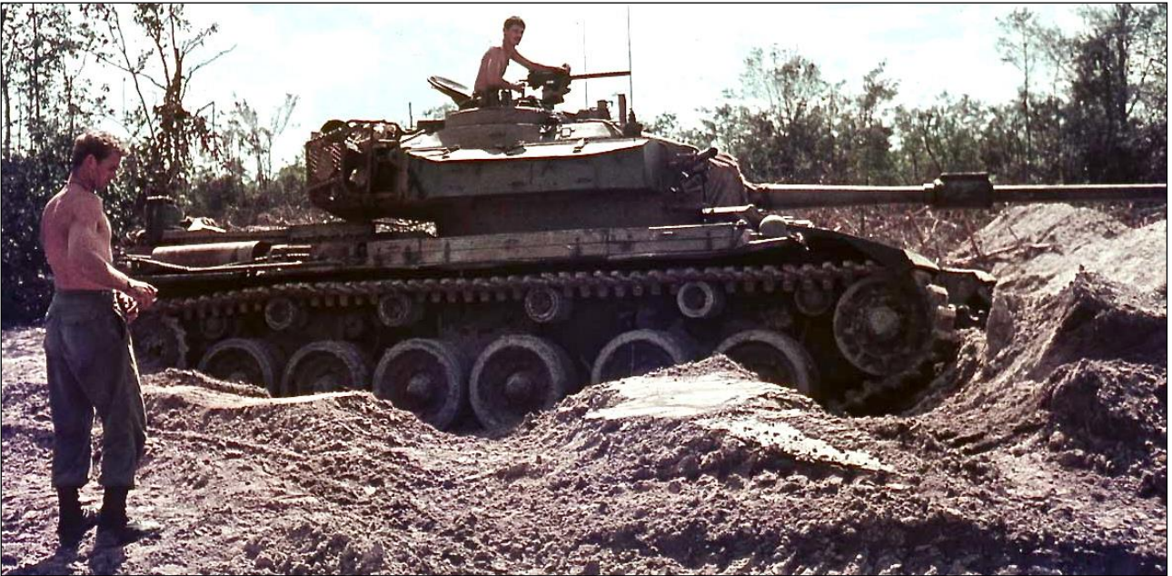
Tank 32A digging itself into the ground to create a forward defensive sand bund 'night position'. Watching on is Sgt Dave Mancer, 11 Platoon, 'D' Company. Sitting on top of tank is Pte John Bryant. During daylight hours the tank would pull back to an 'out of sight' position. (Photo courtesy of John Bryant).
