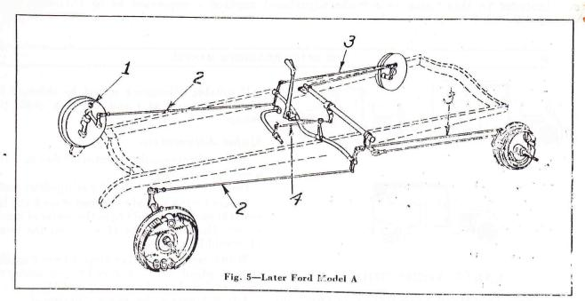
The linkage layout is now as shown in Fig. 5. The construction and adjustment of the service brakes remains the same as on the earlier models.
