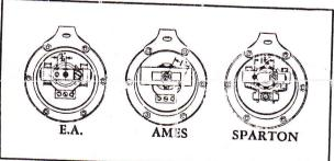
As we previously pointed out in an earlier issue, the Model A Ford horn was manufactured by three suppliers—Ames, A. E., and Sparton—who stamped their name on the cover. Should the cover be missing, it will be necessary to measure the distance between adjusting screw and mounting screw to determine the make of the horn (according to our diagram, left) before attempting to find a replacement, since none of the three covers are interchangeable.
