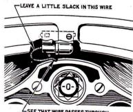
SEE THAT WIRE PASSES THROUGH THIS NOTCH IN INSTRUMENT PANEL
