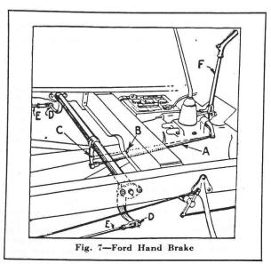
anchorage on the upper band, but this will not be possible if the bands are in the least distorted or are not concentric with the brake drum. Slipping or squeaking may then result.
