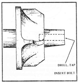
O Place the shaft in a machine lathe and use a 17/64" drill to drill a hole in the centre of the shaft to accommodate a 5/16" brass bolt. The hole should be 1/4" to 1/2" deeper than the proposed bolt length.
