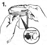
Place the expander in oil ring T groove. Do not overlap ends.
