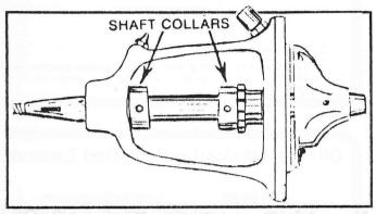
I Got end play or worried that the press-fit impeller may come loose and the fan will demolish your radiator? Buy a couple of 5/8" shaft collars (they look like a thick washer with a locking screw). Fit one behind the front bearing (but not touching the casting) and the other in front of the packing nut (which will be greased by seepage from the packing).
