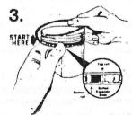
Wind on lower rail with its ends approximately ¼ turn from expander gap and on other side of expander gap to upper rail.
