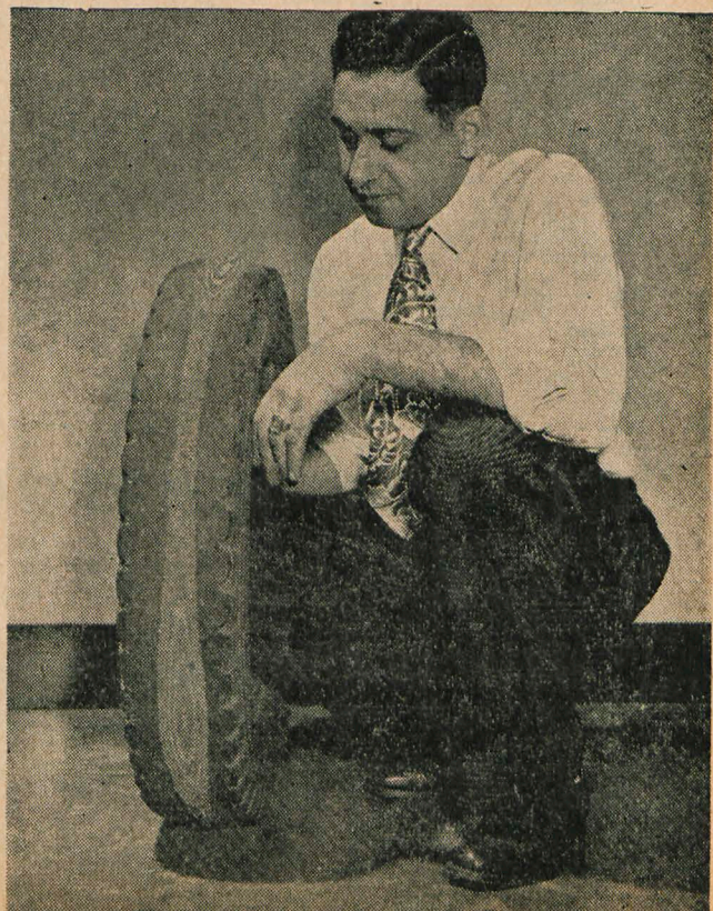
4. This tyre is badly neglected, as can be seen by the excessive wear. What could cause this?
