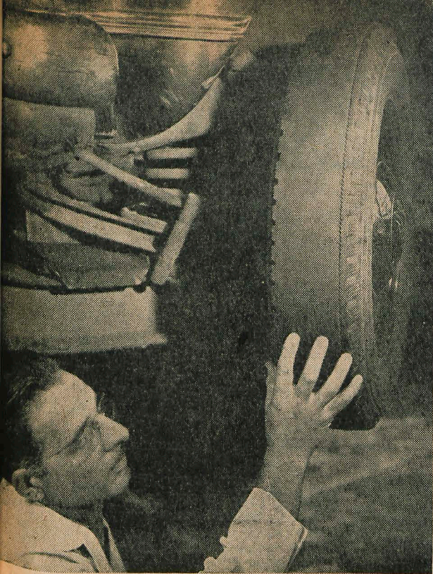
1. Notice how the front tyre is worn with a feathered edge on the inside. What is the cause?
